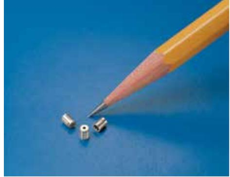
Installation is simple. Press or heat flow the orifice into a plastic hole, narrow end first, until the orifice is flush minimum with the top of the installation hole. Pressing or heat flowing the restrictors into the manifold or fitting provides retention and creates a leak tight seal.
