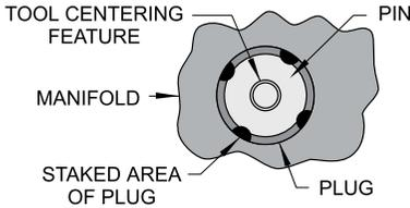
Lee Installation/Staking Tools are available for each Betaplug and part numbers are listed in each section.
