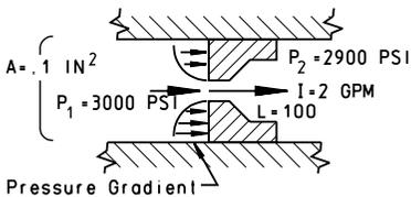
The momentum force of 1lb. in this example must be subtracted from the force produced by static pressure on the plate (of  $0.1 \times [3000-2900] = 10 \text{ lb.}$ ) to give the total force on the piston.
