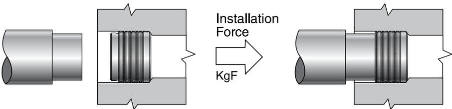
IMH Cartridge Screens use proprietary high strength bonded mesh to provide additional strength and integrity for applications where higher pressures could cause rupture due to the effects of clogging, possibly with catastrophic consequences. The unique design of the Lee Cartridge Screen is engineered to prevent a rupture and instead allow a gradual reduction in flow performance.
