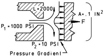
The momentum force of 0.2 lbs. in this example must be added to the force produced by static pressure on the plate ( $0.1 \text{ in.}^2 \times 10 \text{ psi} = 1 \text{ lb.}$ ) to give the total force on the plate.
