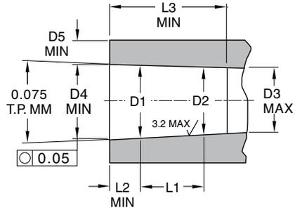
The Lee Company recommends that the Betaplug be installed below the surface of the housing to ensure maximum plug retention capability. The use of coatings or surface treatments in the area of the installation hole where the Betaplug is to be installed is not recommended.
