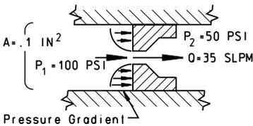
The momentum force of 0.05 lb. in this example must be subtracted from the force produced by static pressure on the plate ( $0.1 \text{ in.}^2 \times [100-50] = 5 \text{ lb.}$ ) to give the total force on the piston.
