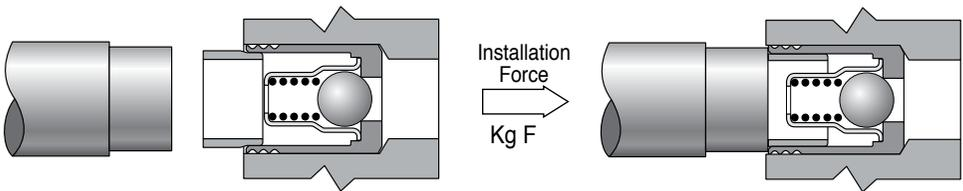
The insert principle eliminates the need for threads and o-rings. Simply insert the component into a drilled hole and drive the expander pin flush to within 0.25mm (0.010") above flush of the insert. The installation tool can bottom on the insert body. Lee Installation Tools are available for each product and part numbers are listed on each page.
