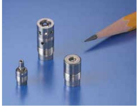
A high quality metal to metal seat limits leakage in the checked direction to no more than 20 sccm of air at 172 kPa (25 psi) differential. The valves are compatible with hydraulic fluids, brake fluids, fuels and oils. Integral safety screen protection is available, (see drawings below).
