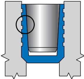
The matching tapers of the Betaplug and its installation hole create a perfect fit, eliminating the need for additional expansion. Since the Betaplug's expansion is precisely controlled by the size of the tapered pin, the amount of expansion and any resulting boss stress is completely predictable.
