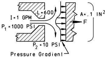
The momentum force of 1.6 lbs. in this example must be added to the force produced by static pressure on the plate (of  $.1 \text{ in.}^2 \times 10 \text{ psi} = 1 \text{ lb.}$ ) to give the total force on the plate.
